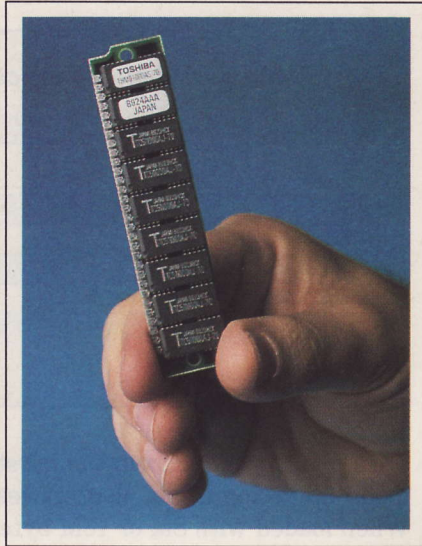
Nine million transistors require very little room when packaged as a 1M×9-bit SIMM (single in-line memory module). The All-Star PC uses 16 of these 70-nsec THM91000AS-70 SIMMs from Toshiba America Electronic Components Inc.
